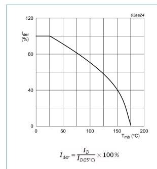
Fig 1. Normalized continuous drain current as a function of mounting base temperature
